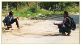
pavement failure, cracks and shoulder condition. These details can be collected through visual inspection and/or with horizontal straight edge and ruler. The data needs to be classified under various headings namely, GOOD, FAIR and POOR with rating assigned to each classification.
